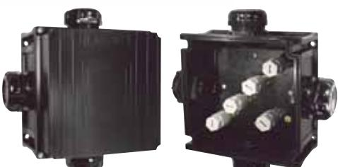
This range is equipped with CRIC increased safety 'e' terminal blocks and cable gland and complies with the 94/9/CE directive (one M40 cable gland maximum per side). All external fastenings are in stainless steel.
