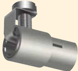
*DXN: a captive pad protrudes into the terminal chamber to protect the strands of the conductors from contact with the tightening screw*
