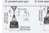
Weight: 7.80kg (70type) 8.80kg (120type) Accessories supplied with the light fittings:
